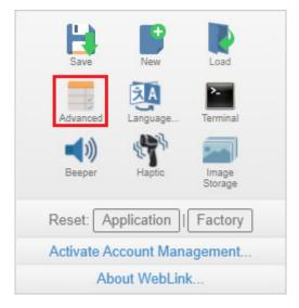
WebLink's Advanced settings allow you to make fine adjustments to individual command parameters in all areas of your reader's functionality: Camera Setup, Communications, Read Cycle, Symbologies, I/O, Symbol Quality, Match String, Diagnostics, Image Storage, and Configuration Database. Many of these commands can be configured directly in the WebLinkhh user interface, but all parameters can be configured and examined in Advanced settings.
