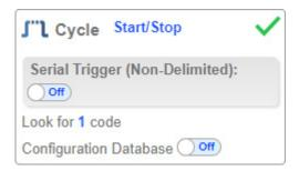
In **Start/Stop** mode, the reader goes into **Continuous Read** mode when you pull the trigger, and exits Continuous Read mode when you release the trigger, or after **1 second** of holding the trigger (by default).
