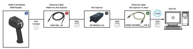
NOTE: Once the reader is connected, If the Ethernet cable ( PoE injector to PC) will be unplugged (on either side), the reader will start beeping to notify the user.
