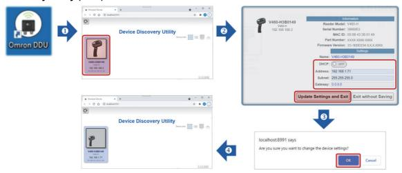
The V460-H's IP Address parameters must match those of the PC's Ethernet adapter.
