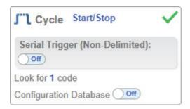
In Start/Stop mode, the handheld goes into Continuous Read mode when you press the trigger, and exits Continuous Read mode when you release the trigger.
