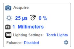
When Time of Flight (found in Advanced Settings > Camera Setup or Advanced Acquire Settings) is enabled or Auto Exposure and Gain (found in Advanced Settings > Camera Setup or Advanced Acquire Settings) is enabled, the A shown on the sun icon and dial icon signifies that Exposure and Gain will be updated automatically based on Time of Flight or Auto Exposure and Gain.
