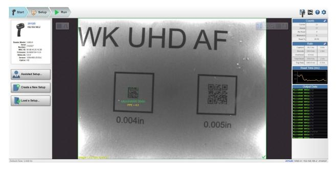
Click the gear icon at the upper right to bring up the **Application Settings** menu. This menu includes several functions: **Save**, **New**, **Load**, **Advanced**, **Language**, **Terminal**, **Beeper**, **Haptic**, **Image Storage**, **Reset Application Settings**, **Reset to Factory Settings**, **Activate Account Management**, and **About WebLinkhh**.
