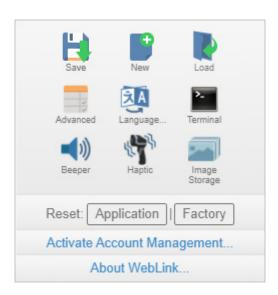
Click About WebLinkhh to display your current WebLinkhh version, Reader Model, Serial Number, Part Number, MAC ID, Sensor, Firmware version, Boot version, Browser, Operating System, and Screen Resolution.
