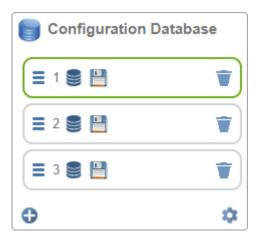
...will remove the first and select the second configuration database index. However, all database indexes above shift down, so the second becomes the first and the third becomes the second.
