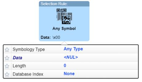
For the image below, without any selection filter and with the number of codes set to five, all codes will be decoded and output.
