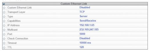
Custom Ethernet Link is intended for advanced users. This feature permits the establishment of a connection to the reader on any port, using the protocols UDP/IP, TCP, and Multicast on a specified port. A bi-directional communication configuration is available to send commands to the reader, obtain barcode output data, or form a single direction of communication, i.e. sending commands to the reader only, or receiving barcode data from reader only, without having both directions open.
