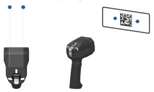
The aiming dots are smaller when the V460-H is closer to the symbol and larger when it is farther from the symbol. Scan symbols with smaller bars or elements (mil size) more closely, and those with larger bars or elements (mil size) more distantly.
