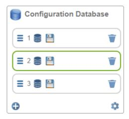
...clicking **add** will insert a new database index (database index 3) after database index 2, and database index 3 will be selected.
