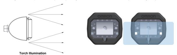
Torch Illumination cannot be used in combination with Dome Illumination or Low Angle Illumination.
