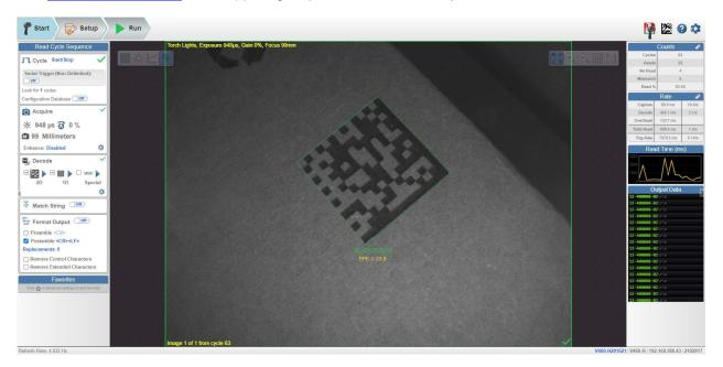
The **gear icon** at the upper right brings up the **Application Settings** menu. This menu includes several functions: Save, New, Load, Advanced, Language, Terminal, Beeper, Haptic, Image Storage, Reset Application Settings, Reset to Factory Settings, Activate Account Management, and About WebLinkhh.
