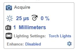
When Time of Flight (found in Advanced Settings > I/O or Advanced Acquire Settings) is enabled or Calculate Exposure and Gain (found in Advanced Settings > Read Cycle or Advanced Acquire Settings) is enabled, the A shown on the sun icon and dial icon signifies that Exposure and Gain will be updated automatically based on Time of Flight or Calculate Exposure and Gain.
