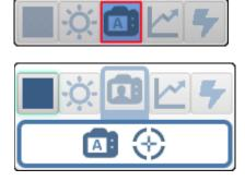
The button turns **Autofocus on** or **off**. This button is only available when the reader is in **Continuous Mode (Presentation)**. The reader's focus settings, defined in the **Acquire** section of the **Setup** interface, are applied to the image when Autofocus is on. The focus setting becomes read-only when Autofocus is on.
